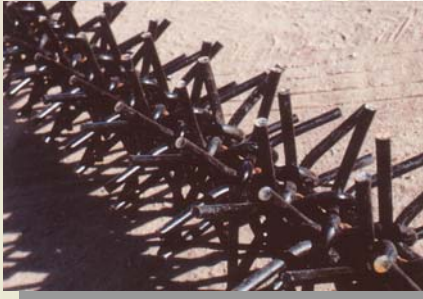
Offset tines disturb more soil leaving a smooth seedbed.
