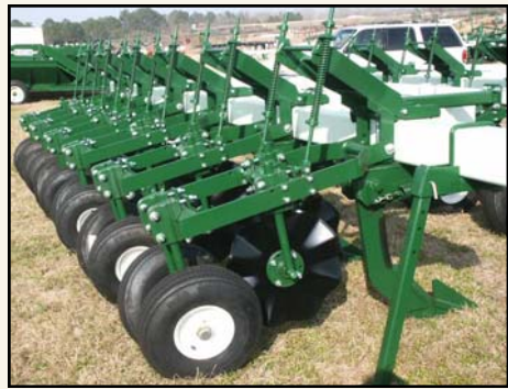
Waffle Coulters (2) with Rubber Tire Press Wheels:
