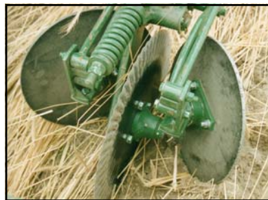
Optional KMC Row Cleaner removes heavy residue from the row allowing row tillage components to run in clean soil. Unique parallel linkage design allows row cleaner to float and remove residue not soil. Adjustable width.
