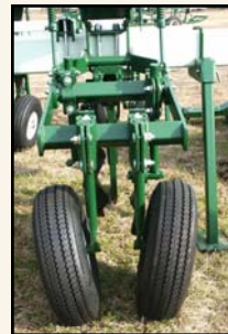
Minimum till and close the slot made by the shank.
