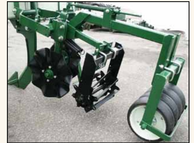
Waffle Coulters (2), Crumbler, and Roller:
