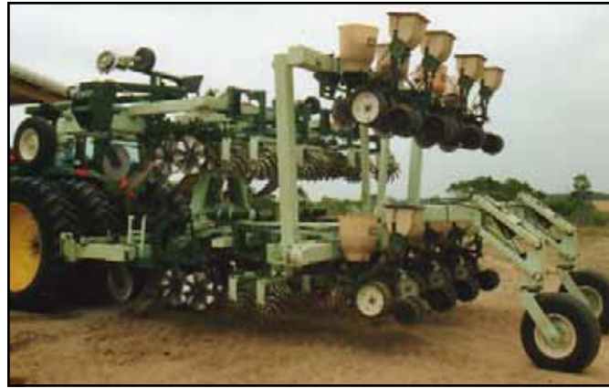
Optional Lift Assist Wheels for carrying seed planter with Rip Strip.
