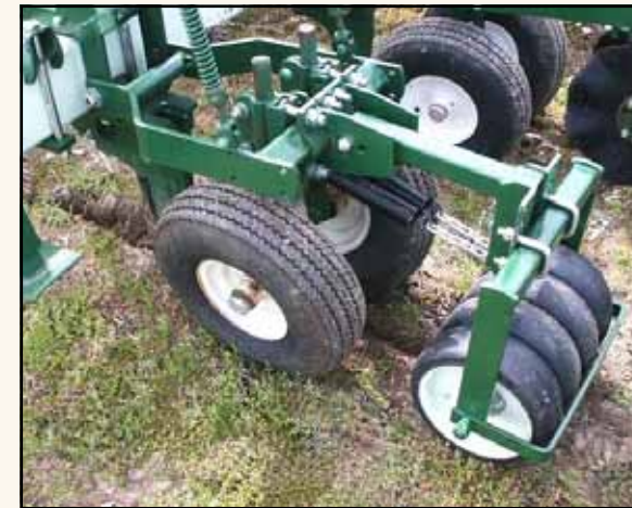
Rubber Tire Press Wheels with Roller:
