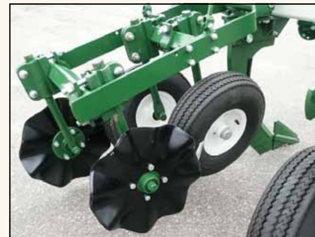
Rubber Tire Press Wheels with Waffle Coulters (2):
