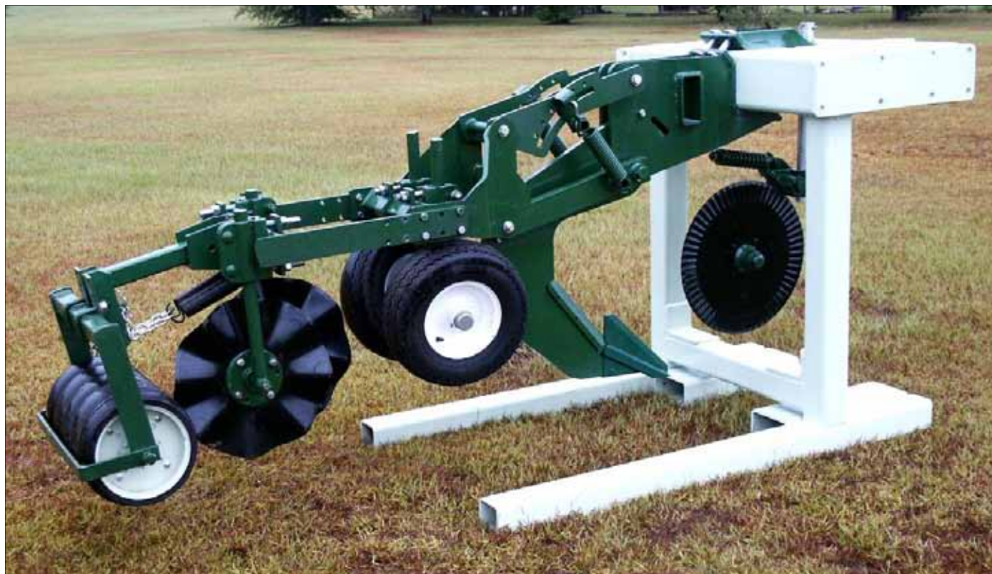
Rubber Tire Press Wheels with Waffle Coulters (2) and Roller: Close slot, minimum till and firm the soil.
