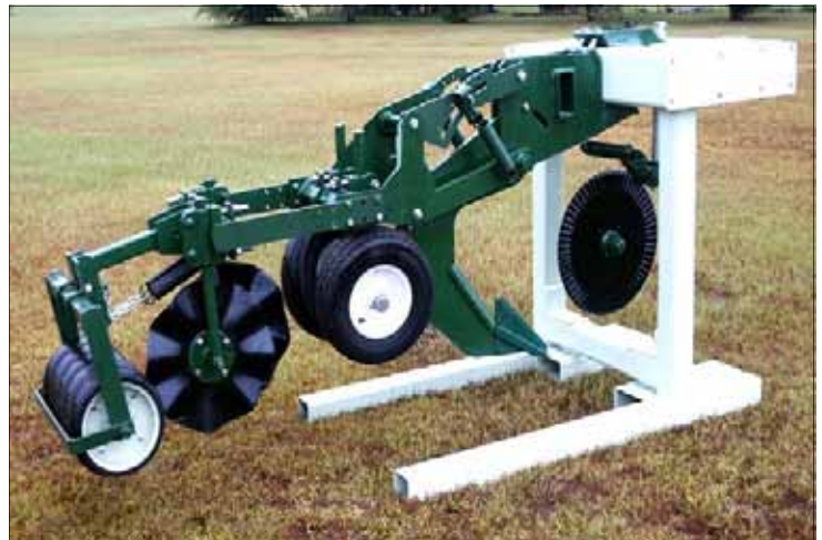
Rubber Tire Press Wheels with Waffle Coulters (2) and Roller: Close slot, minimum till and firm the soil.
