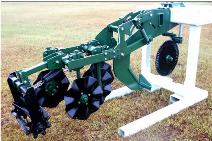
Waffle Coulters (4) with Crumbler: Additional tillage in tougher soils.
