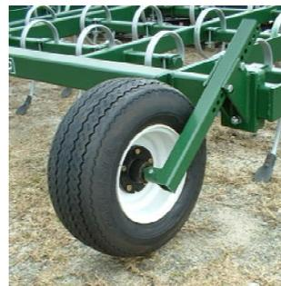
Optional gauge wheels (8 x 8 or 8 x 10) are front mounted to prevent interference with soil mixing activity.
