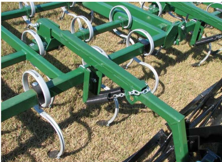
Maximum soil stirring action and excellent trash clearance is provided by the special arrangement of strong, high-quality S-tine shanks on the implement. Our shanks are constructed from 3/8" x 1 1/4" spring steel with 16" mounting height. Also included are long-wearing 1/4 x 2 3/4 sweeps.
