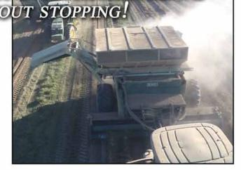
Two full baskets can be EMPTIED INTO THE DUMP CART VIA HYDRAULIC CONVEYOR WHICH IS CONVENIENTLY CONTROLLED FROM THE TRACTOR CAB.
