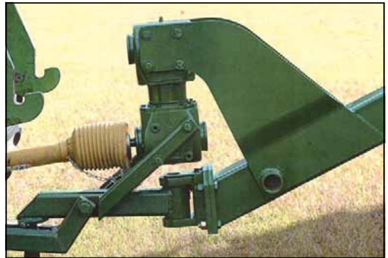
Double Gear Box allows smooth type turns. Standard on both models.
