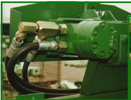
Larger sifter and leveler motors (34% larger on sifter, 45% larger on leveler). All motors mounted inboard for more side clearance.
