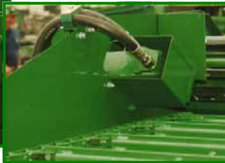
Larger sifter and leveler motors (34% larger on sifter, 45% larger on leveler). All motors mounted inboard for more side clearance.
