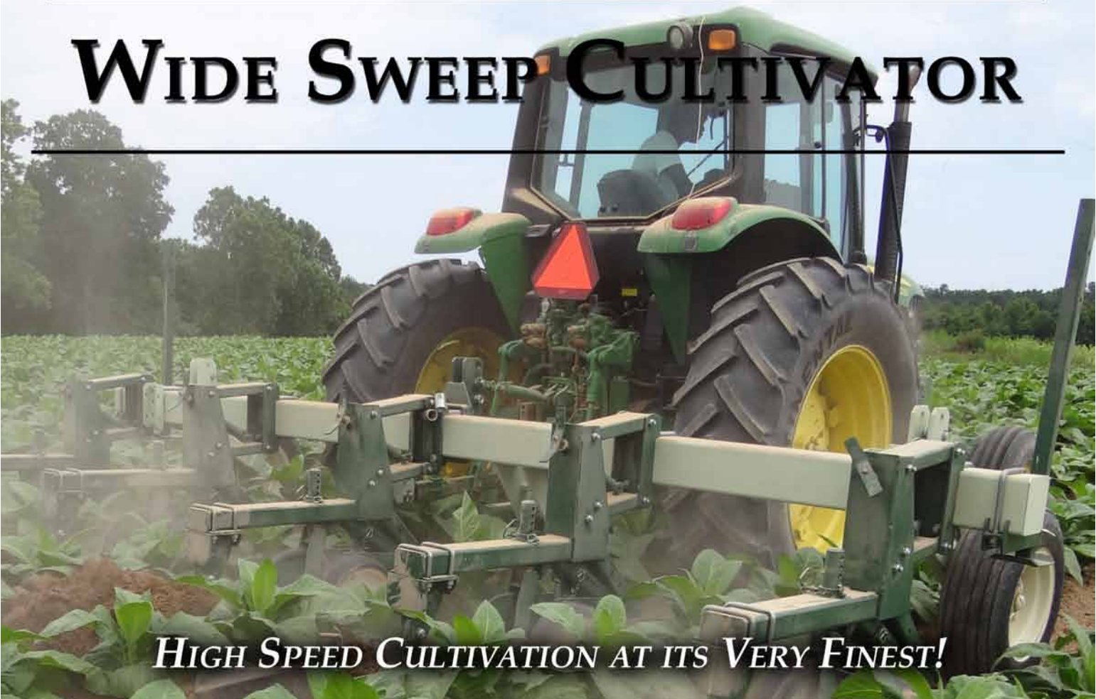
FERTILIZER ATTACHMENT-GROUND OR HYDRAULIC DRIVE- 500 LB HOPPERS
