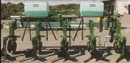
FERTILIZER ATTACHMENT-GROUND OR HYDRAULIC DRIVE- 500 LB HOPPERS
