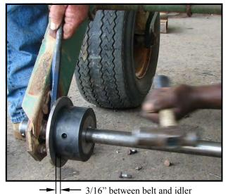
Place 1/4 x 3 1/8 key in shaft and slide front flange idler onto the key. This may require using a hammer to position part into place. Once part is in the correct position tighten the setscrews over the key and one on the shaft with the proper size allen wrench as shown below. Screw in setscrew tightly to score key or shaft, then back off a half a turn. Seat down tight on shaft making sure setscrews cut into shaft. Torque to 27 ft lbs. Leave approximately 3/16" between edge of belt and idler.
