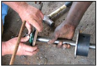
Now place front flange idlers and center front idler on front shaft as shown in the drawing above. Assemble 3 hole flanges around bearing to block idler, with collar of
