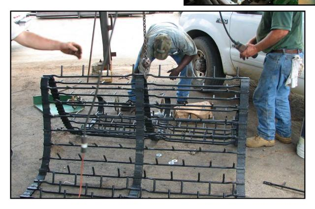
Roll out belt flat on ground. Using a hoist, lift conveyor over the rattler frame and lower it down on to the rear sprockets and front idlers. Make sure that the block idler is loose enough to help you attach the belt together.
