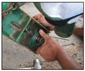
bearing facing outward. Now slide bearing and idler onto the shaft and slide into place on the rattler side frames.
