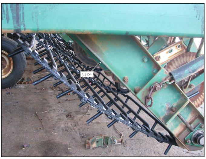
Run belt loose. **<u>DO NOT</u>** over tighten. Leave same amount of droop on each side, 3 1/2" below rattler frame between knocker wheel locations.
