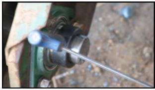
When shaft is in the correct location tighten the setscrew in collar to lock bearing to shaft.
