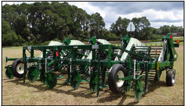
8 ROW: MAXIMUM CAPACITY DIGGING. ALLOWS EIGHT ROWS TO BE INVERTED UNIFORMLY AND SPACED EVENLY. *BELTED MODEL SHOWN.
