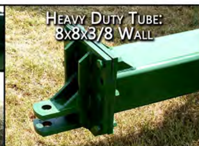
REINFORCED FRONT TO REAR FRAME SUPPORT
