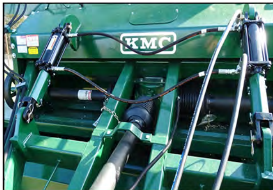
NEW T-BOX DESIGNED FOR COMBINE TO BE DRIVEN OFF BOTH SIDES
