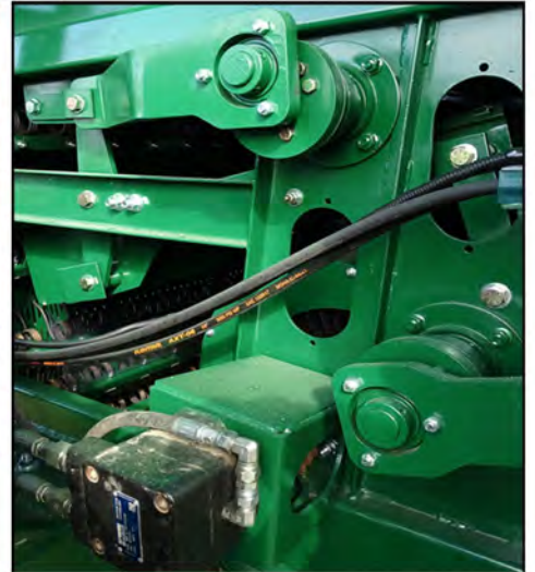
HYDRAULIC SEPARATOR FAN DIRECT DRIVE OPTION (NOBELTS)
