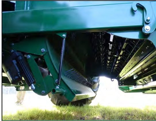
#1 CONCAVE SWINGS OPEN WITH QUICK RELEASE LATCHES
