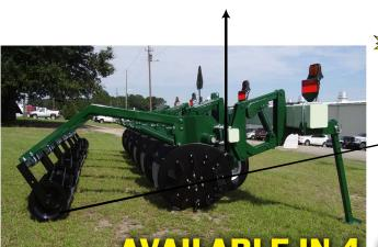
**CRUMBLERS** HELP SEPARATE SOIL FROM ROOT BALL AND SMOOTH AND LEVEL SOIL SURFACE.
