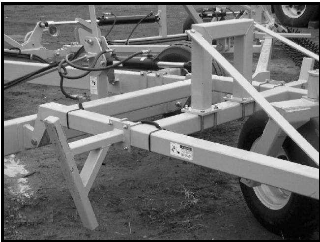
Decals, Falling Tail Wing Hazard Located on Tail (Both Sides)
