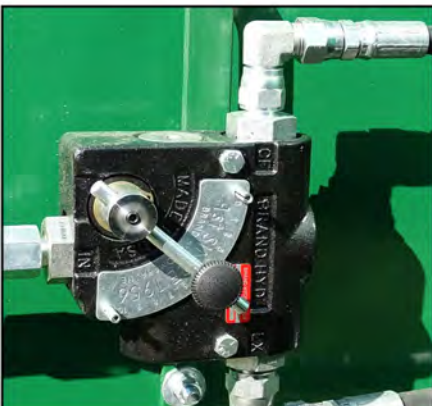
NEW VARIABLE FLOW VINE SPREADER CONTROL
