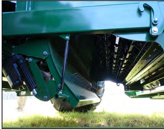
#1 CONCAVE SWINGS OPEN WITH QUICK RELEASE LATCHES
