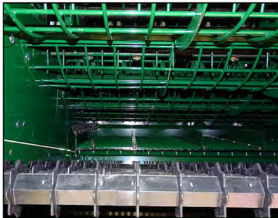
- LARGER CONCAVE OPENINGS - HEX ROLLERS ADDED TO CLEANING SYSTEM
