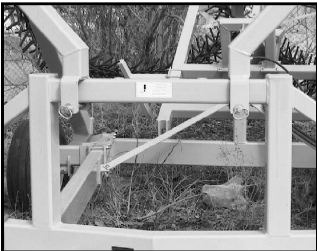
Decals, Transport Locks Located on Front Wing Mount
