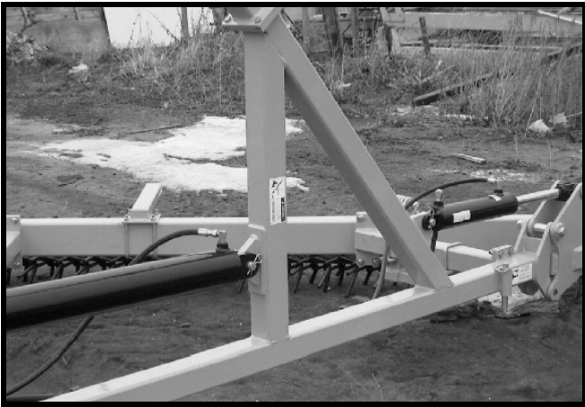
Decals, Falling Wing Hazard Located on Front Beam (Both Sides)
