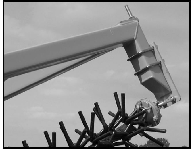
Rear Bearing Housing Height Adjustment
