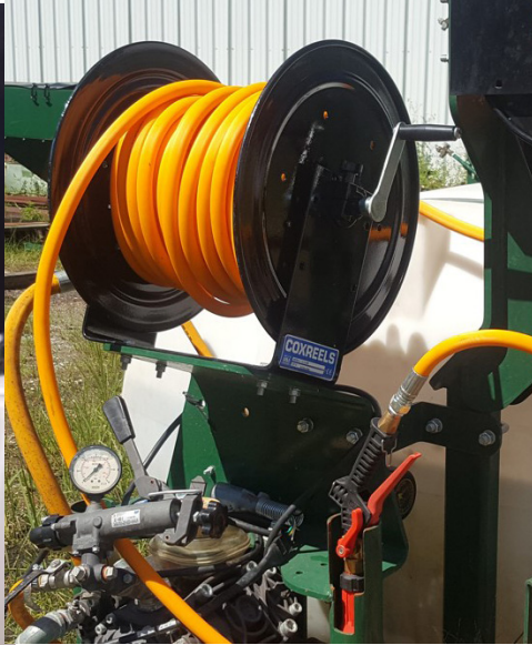
Optional Front High Capacity Hose Reel (Manual) w/ Driver Knockdown-Cool Cell Spray Gun
