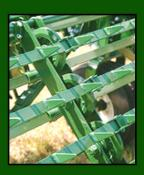
Highly-functional 3-wheel dirt knocker assembly can be adjusted to remove soil, rocks, and other debris for cleaner windrow conditions. Replaceable dirt knocker pads on rattler bars.
