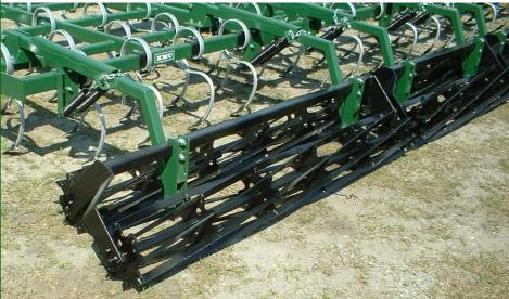
Heavy-duty crumbler attachments are hinged to middle of mainframe for reduced stress when lifting. Spiral strips are made of 1/4" x 1 1/4" C1045 carbon steel for toughness and long wear life. Outside Re-enforcement Crumbler Plates are made of the same type of material. A special linkage is designed to give the crumblers a more floating action for increased performance on unlevel soils. It's Equipped with non-regreaseable Tri-Ply sealed bearings.
