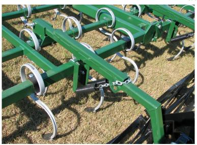
Maximum soil stirring action and excellent trash clearance is provided by the special arrangement of strong, high-quality S-tine shanks on the implement. Our shanks are constructed from  $3/8" \times 1 1/4"$  spring steel with 16" mounting height. Also included are long-wearing  $1/4 \times 2 3/4$  sweeps.
